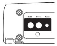
The A1400's "+12VDC" and "Ground" connections are designed to accept 4 AWG power wire. 4 AWG is a minimum power wire size for this amplifier.
